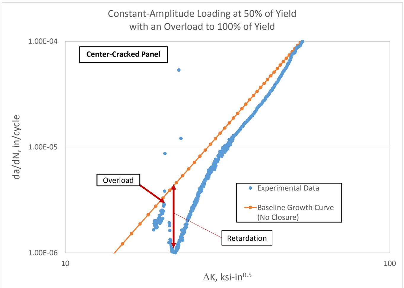
FIGURE 2. Fatigue crack growth data for a carbon steel equivalent to API 5L-X46.
