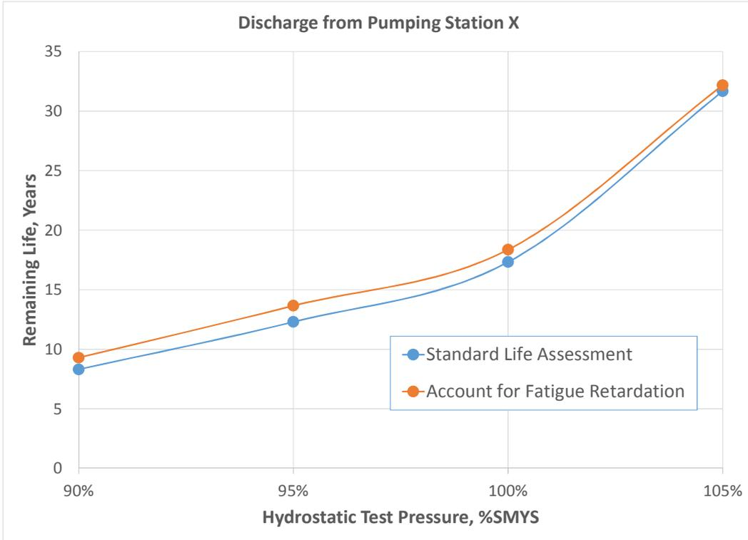
FIGURE 10. Effect of fatigue retardation on remaining life at a pumping station discharge.
