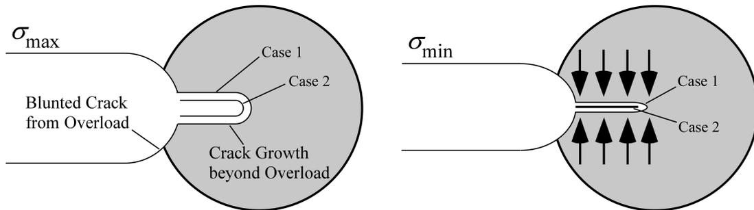
FIGURE 9. Crack propagation following an overload. In order for closure to occur at or above  $\sigma_{\min}$ , compressive residual stresses must overcome crack blunting at  $\sigma_{\max}$ . Consequently, crack closure behavior is a function of the magnitude of both the overload and the subsequent maximum stress.
