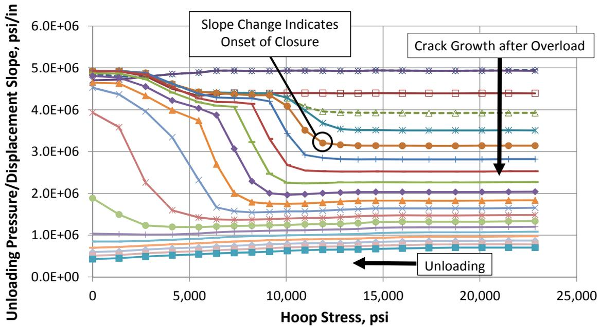
FIGURE 6. Unloading pressure/crack opening displacement slope at various crack sizes following a hydrostatic test to 100% SMYS.
