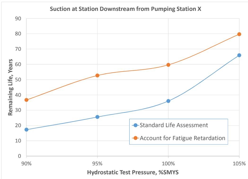
FIGURE 11. Same as Fig. 10, but at the suction of the pumping station downstream from Station X.
