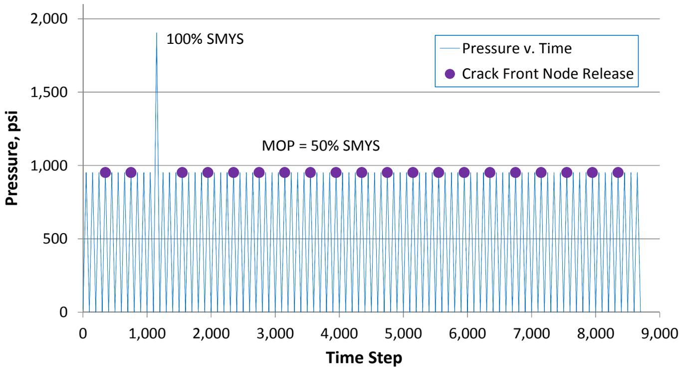
FIGURE 4. Load history for a typical finite element simulation. A pressure spike to 100% SMYS was preceded and followed by constant amplitude cycling between 0 and 50% SMYS in this example.
