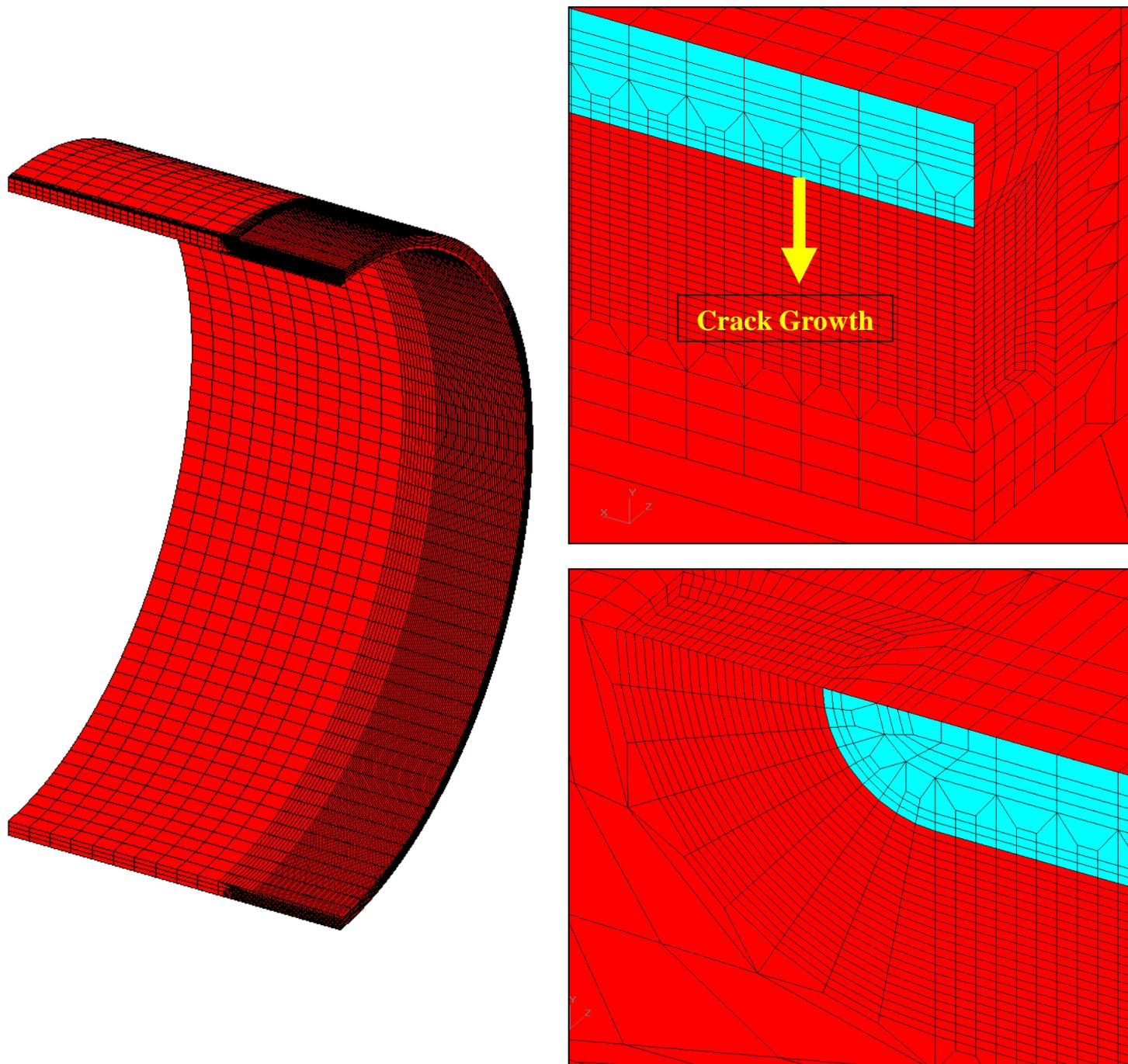
FIGURE 3. Quarter-symmetric finite element model to simulate fatigue retardation.
