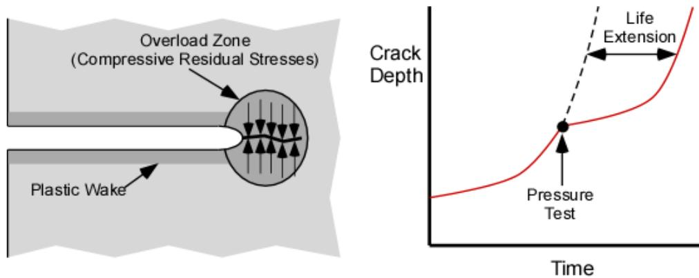
FIGURE 1. Crack closure mechanism for fatigue retardation following a pressure test. The overload generates a zone of compressive residual stresses at the crack tip, which results in slower fatigue crack propagation due to crack closure.
