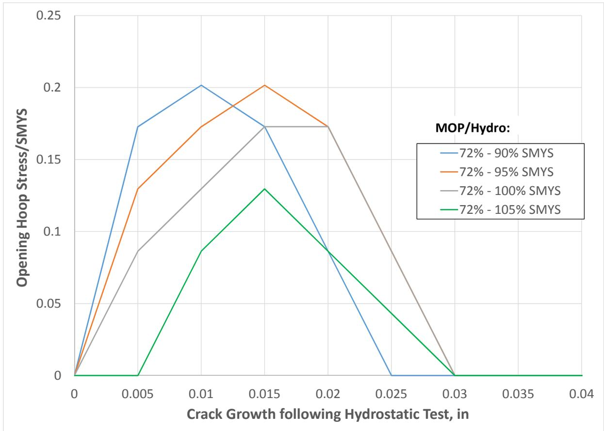
FIGURE 7. Crack opening stress following a hydrostatic test.
