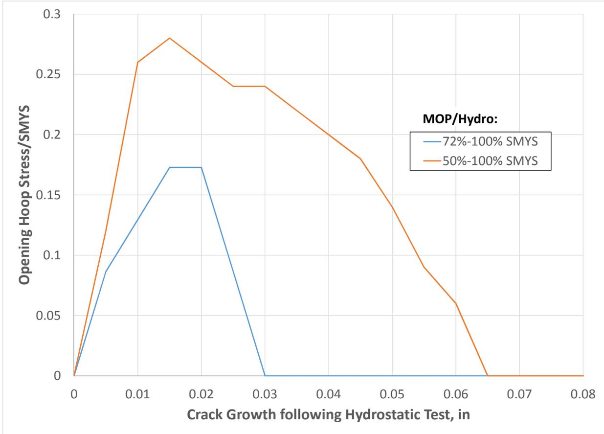
FIGURE 8. Effect of MOP following a hydrostatic test on crack closure behavior.
